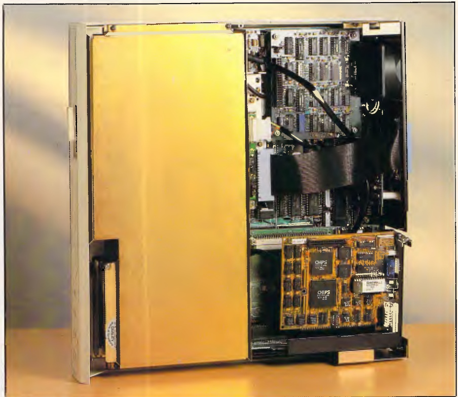
The main PCB is large and occupies all the available floor space
